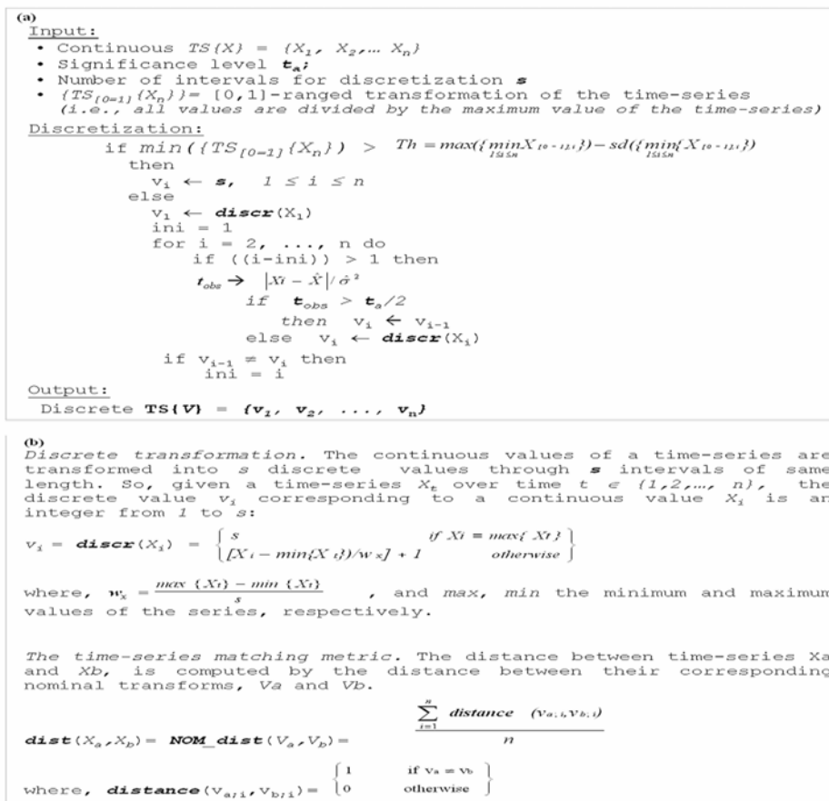
Fig. 2. Time series nominalization: (a) the Qualitative dynamic discretization algorithm; and (b) computation and assignment of discrete values.
