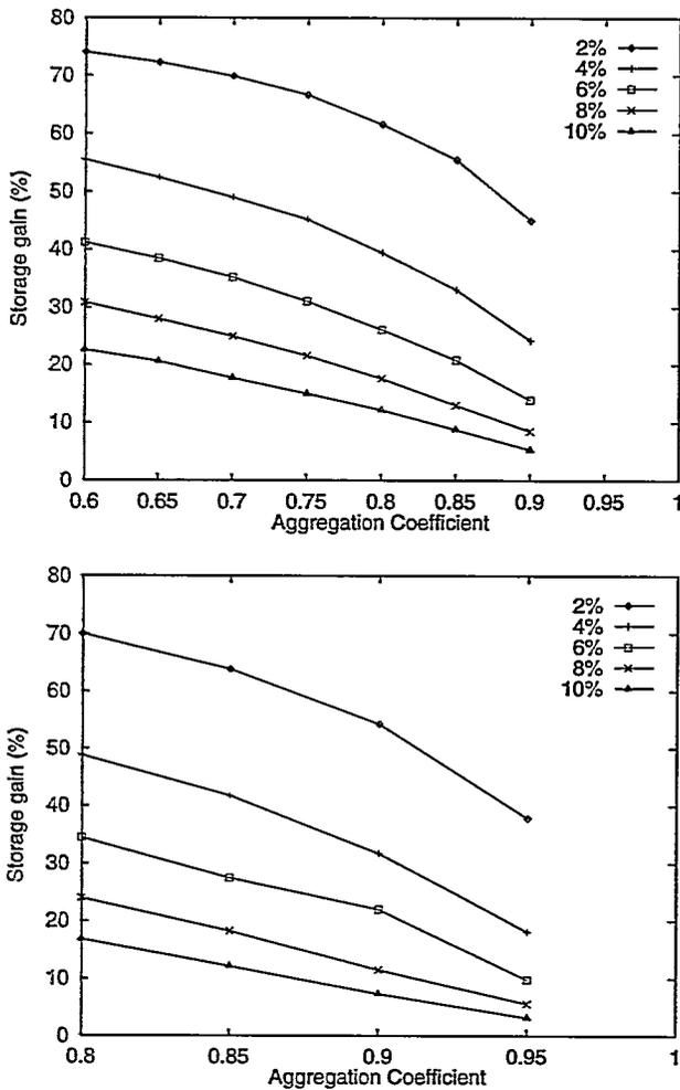
Figure 5: The storage gain as a function of aggregation (obtained during the second experiment), for various change percentages. The images were 60% black (above) and 80% black (below).
