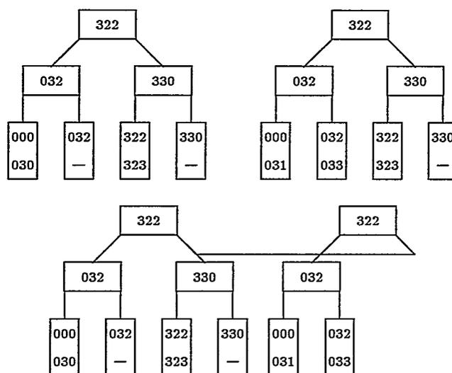
Figure 2: Two  $B^+$ trees storing linear quadtree codes and the corresponding linear overlapped structure.
