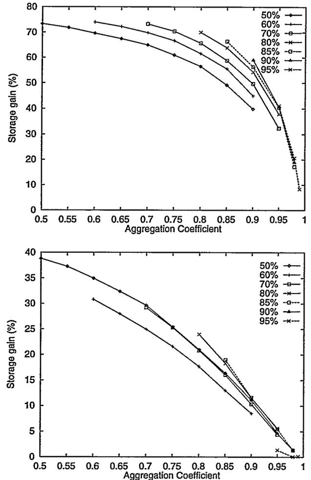
Figure 6: The storage gain as a function of aggregation (obtained during the second experiment), for various black probabilities. The change percentage was 2% (above) and 8% (below).
