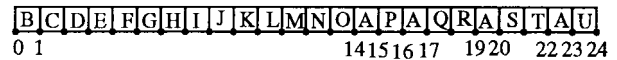
Fig. 11. Server schedule with period 25 and information items \{A, B, \dots, T, U\} .
