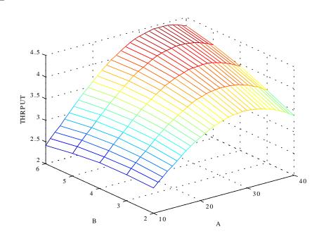
Response surface for **THROUGHPUT** when cpu speed: 0.012 disk speed: 0.028 n of disks: 1
