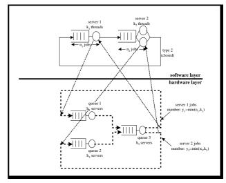
Figure 1: A two-layer queuing network with simultaneous resource possession
