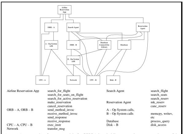
**Figure 1** A structured performance model of a CORBA based airline reservation system and some of the services provided by each one of the model's components
