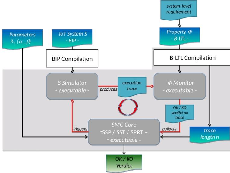
Figure 3: Architecture of the SMC-BIP tool for statistical model checking (source: SMC-BIP website<sup>1</sup>)
