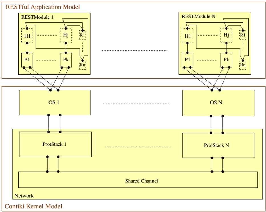
Figure 6: BIP model structure for Contiki WPAN systems
