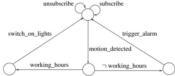
Figure 11: State flow for motion detection by the zone-controller (alarm triggered in non-office hours)
