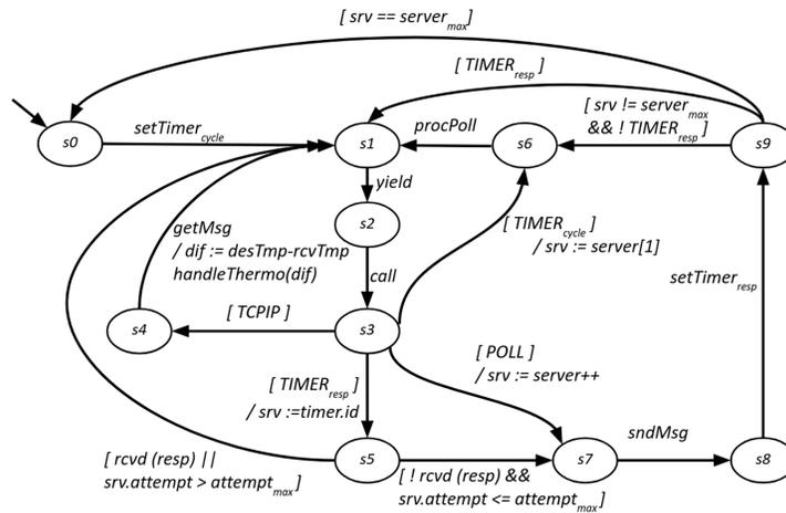
Figure 13: Client process of the building automation application
