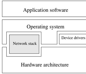
Figure 1: Typical SW/HW architecture of IoT node
